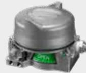
The stainless steel version of the explosion proof Axiom AX is an optimum solution for standard on-off applications. It is a discrete on-off valve controller that combines a solenoid valve and proximity switches into one integrated package. The advanced position sensing system of Axiom offers reliable long-life performance with convenient push-button settings. The internal pneumatic valve has high tolerance to dirty air and it enables perfect operation in demanding off-shore environment.
