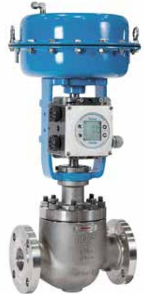
The spring return VD-series diaphragm type linear actuators are designed for use in both modulating control and on-off service. These actuators offer an extremely long cycle life and are well suited to operate linear valves with small to medium thrust requirements.
