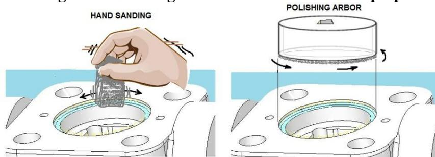
7. **CLEANLINESS** – clean surfaces with a mild degreaser and lint-free cloths to remove any grease or residue, or any loose grit from sandpaper before attempting to install the laminate seals.
