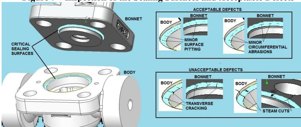
6. Increase the surface roughness of both the body and bonnet critical sealing surfaces by **SANDING** using 120-grit sandpaper – or rougher as needed – using the following methods:
