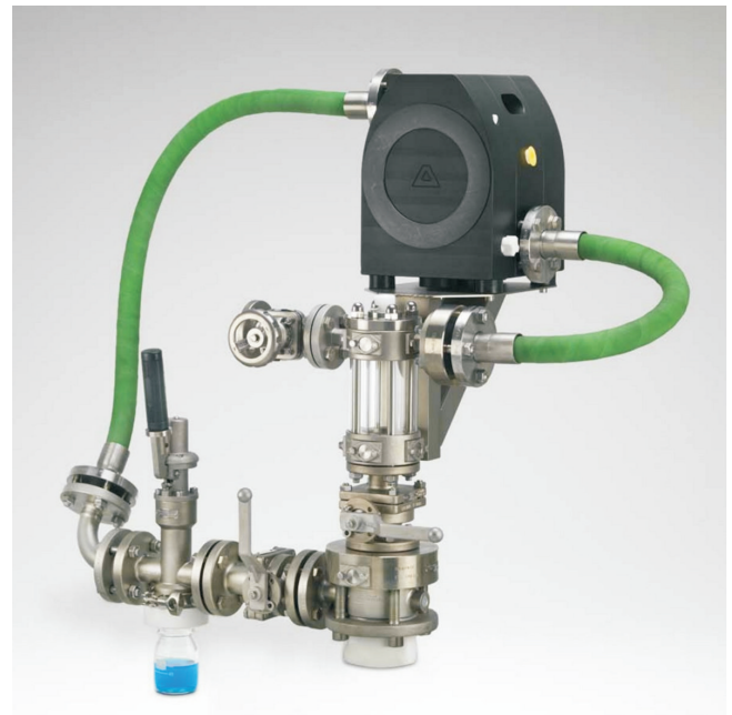
SRS-P-P Reactor Sampling System, with diaphragm pump Sampling by means of forced circulation via Sampling Valve Flanged/adaptor into lab bottle.
