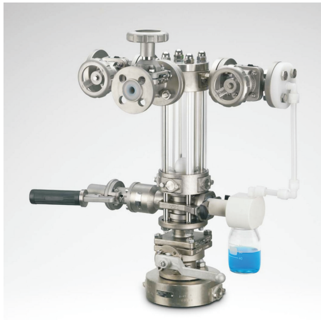
SRS-P Reactor Sampling System, manually Sampling via Sampling Valve Wafer/adaptor 90° into lab bottle, incl. gas return piping.
