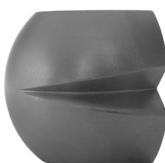
Reduced  $C_v$  trims are available on the DN25/1" valve to control very low flows with high accuracy. The narrow orifice is a selfflushing design because the trim orifice is continually increasing.
